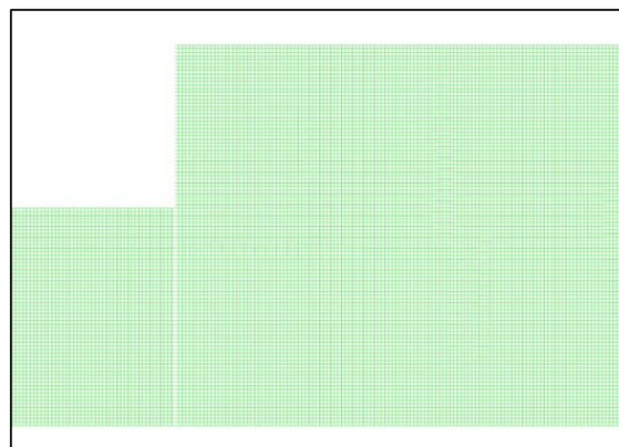
Figure 11. Magnified view of sudden pipe expansion mesh.
